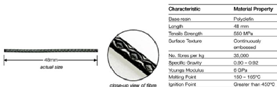
Fig41: Characteristics of polymer threads (source Dez Ab 2011)
