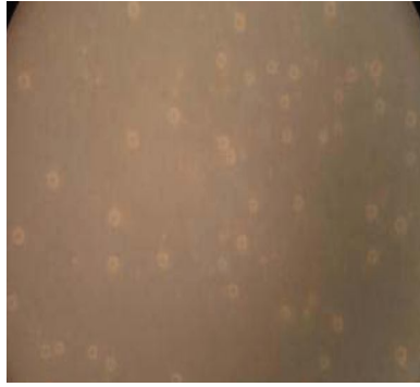
Fig.6-microscopic air bubbles inside the nano-composite
