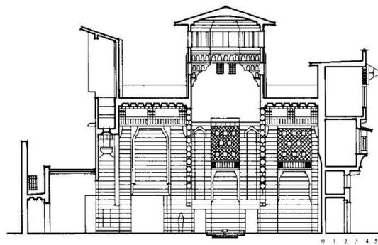
Figure 3. The singular Egyptian Malqaf developed by Qaouf Mohebodini Ashafi Almavaghi, the main Malqaf of Alsouhami residential unit in Cairo (Bahadori Nejad, Mahdi, Dehghani, Alireza, 2008).
