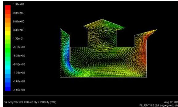
Figure 9. Y directed velocity vectors of Malqaf
