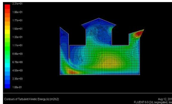
Figure 10. Counters of Kinetic turbulent energy vectors of Malqaf
