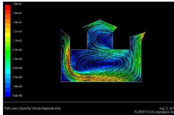
Figure 11. Airflow lines of Malqaf
