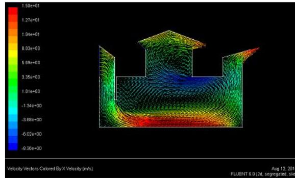
Figure 8. X directed velocity vectors of Malqaf
