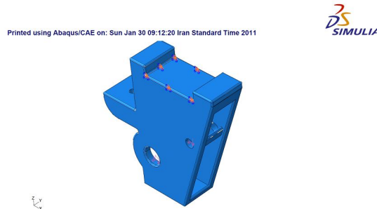
Fig 5. The opener chassis layout supports and loads in Abaqus.
