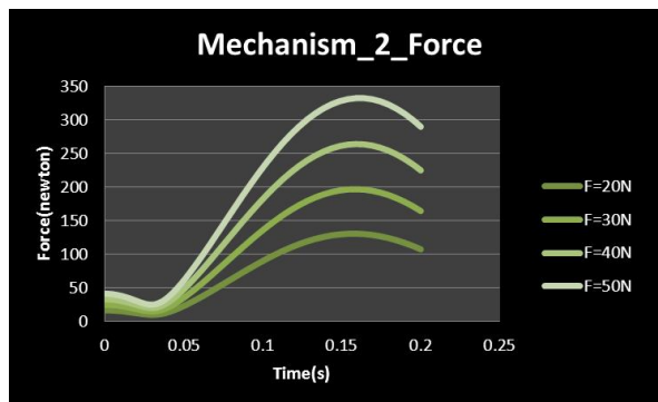
Fig 7. Loads on the second mechanism in four different status of spring deformation.
