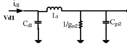
Fig.5. The first inter-stage equivalent circuit.
