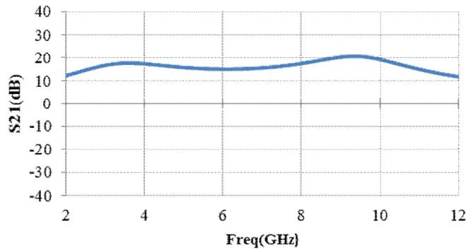
Fig.8. The S21 gain of the design.
