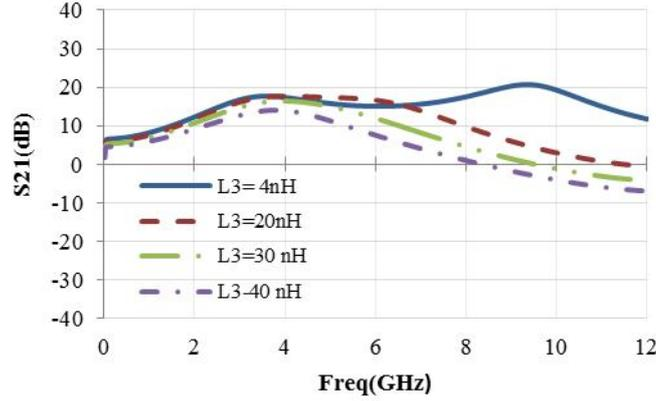
Fig.4. The effect of changing  $L_3$  on gain
