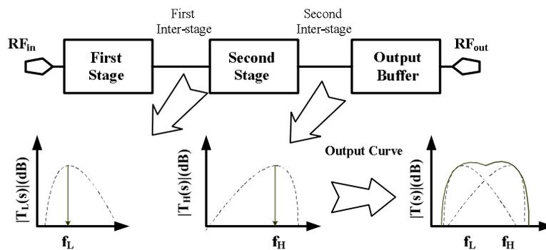
Fig.2. Stagger tuning technique.
