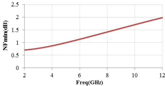
Fig.9. Minimum noise figure of the proposed LNA.
