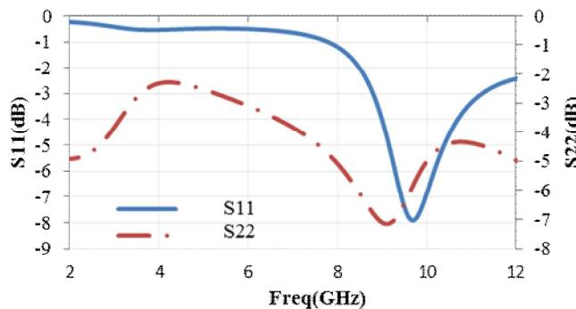
Fig.11. S11 and S22 of proposed LNA.
