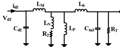
Fig.6. The second inter-stage equivalent circuit.
