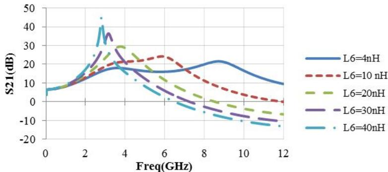
Fig.7. The effect of changing  $L_6$  on high-band resonant frequency
