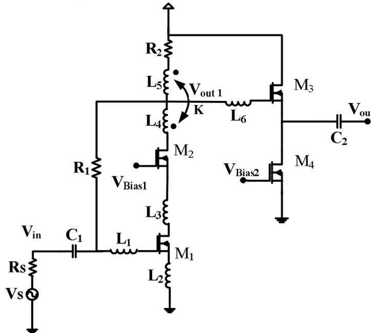
Fig.1. The proposed UWB LNA schematic.
