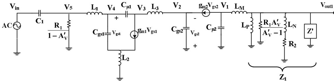
Fig.3. The equivalent circuit model of the cascode stage of the proposed UWB LNA.
