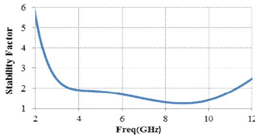
Fig.10. Stability factor of the proposed LNA.
