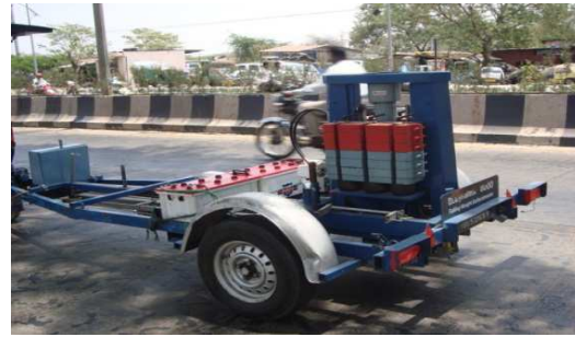
Fig. 6: FWD Test Carried on Study Road
