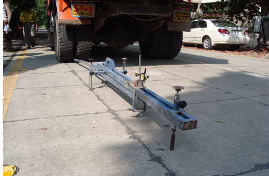
Fig.1: BBD Test in Progress
