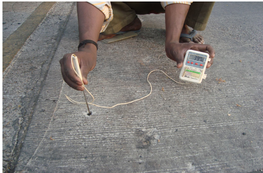
Fig.3: Measuring Pavement Temperature (Inside)
