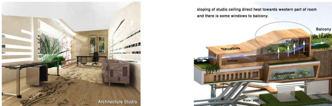
Fig.13.The effect of ceiling slop on ventilation.
