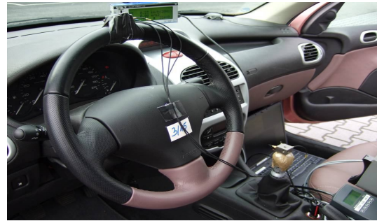
Fig.10. The place of sensors (on the knob & steer)
