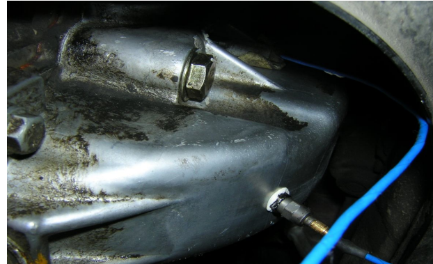
Fig.11. The place of sensors (on the gearbox cover)
