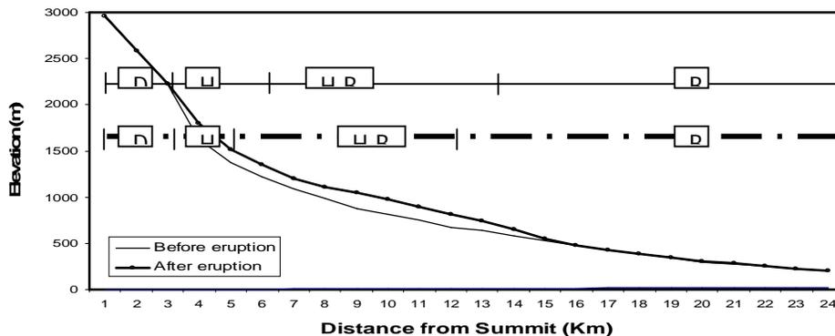
**Figure 7: The change of river slope before and after 2010 eruption**
