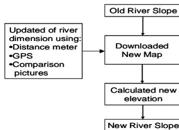
Figure 6: Calculation step of new river slope
