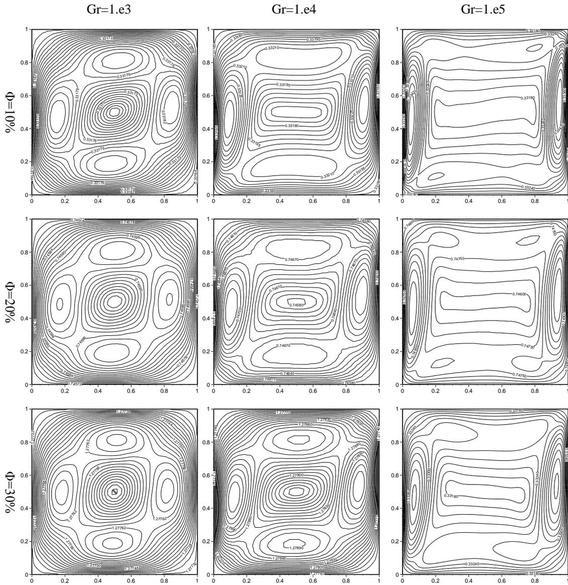
Figure (7)- Effective thermal conductivity enhancement contours for various volume fractions
