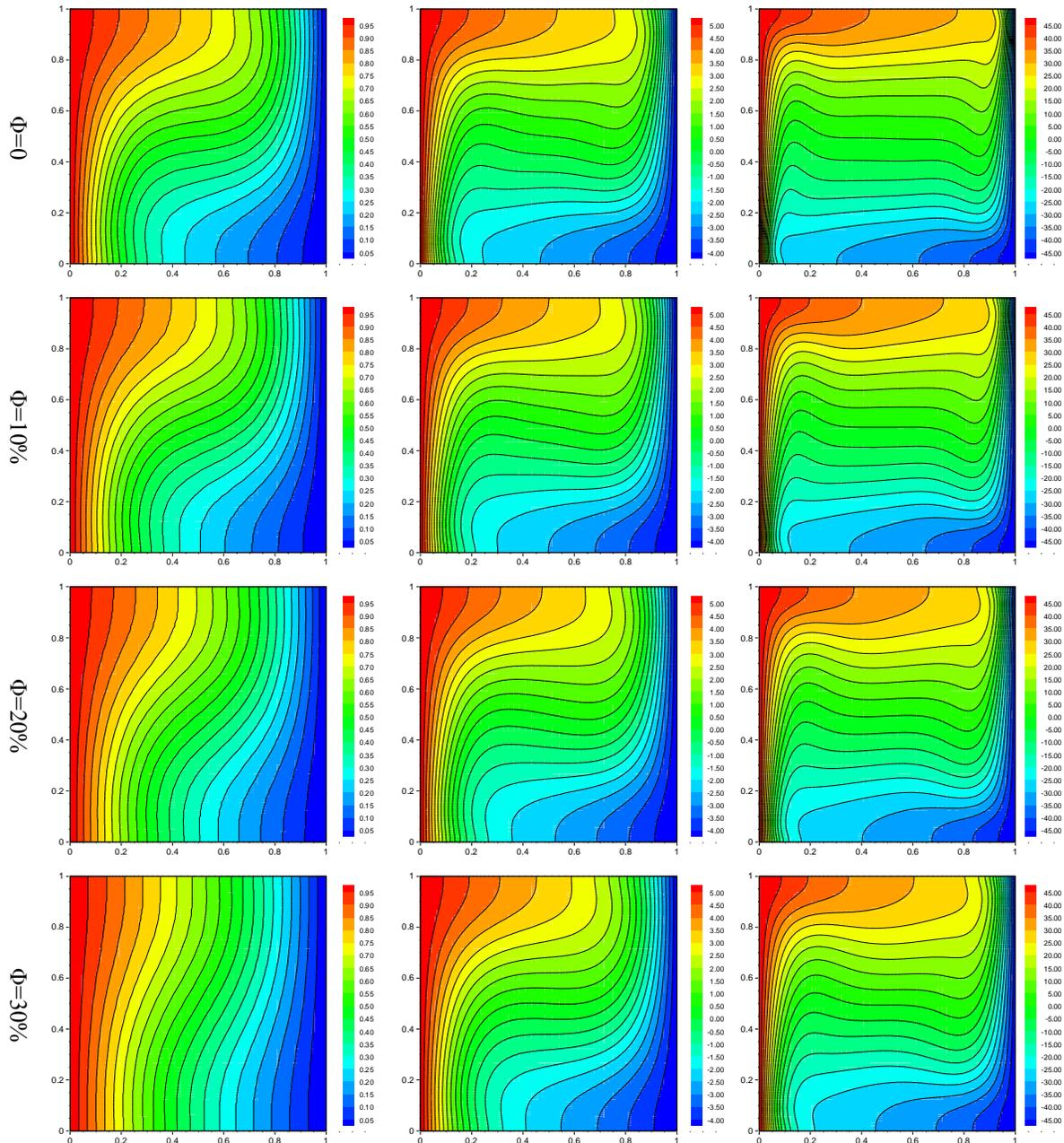
Figure (6)- Isotherms plots for Cu-water nanofluids at various Grashof numbers and volume fraction
