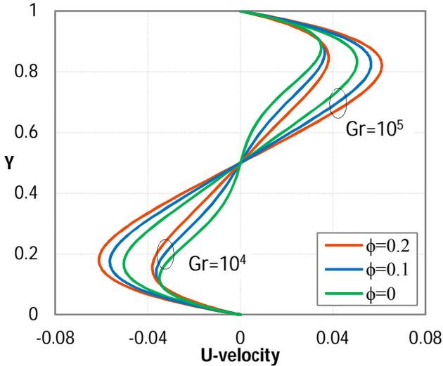
Figure (9)- Comparison of the U-velocity profiles between nanofluid and pure fluid for various Grashof numbers
