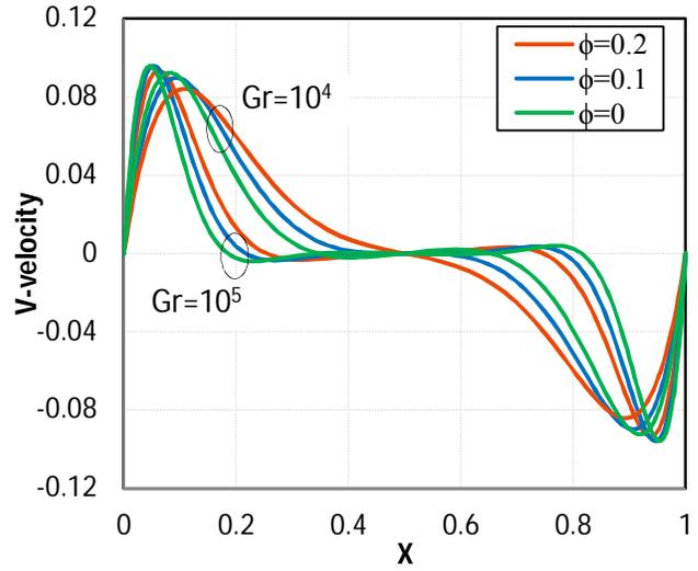
Figure (10)- Comparison of the V-velocity profiles between nanofluid and pure fluid for various Grashof numbers
