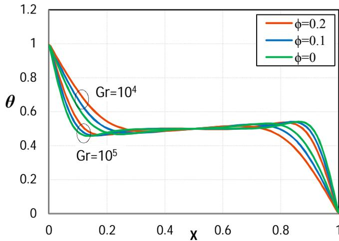
Figure (11)- Comparison of the temperature profiles between nanofluid and pure fluid for various Grashof numbers
