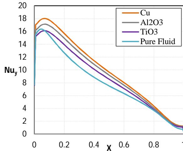
Figure (13)- Variation of local Nusselt number along the hot wall for different nano-particles at  $Gr=10^5$  and  $\phi=0.2$ .
