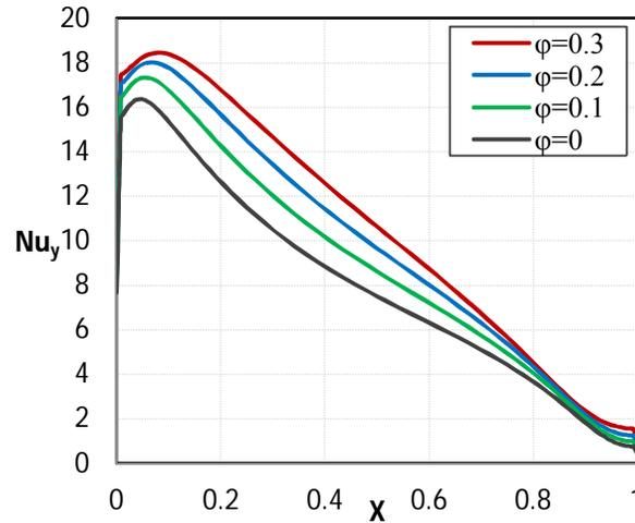
Figure (12)- Variation of local Nusselt number along the hot wall for Cu -water nanofluid at  $Gr=10^5$ .
