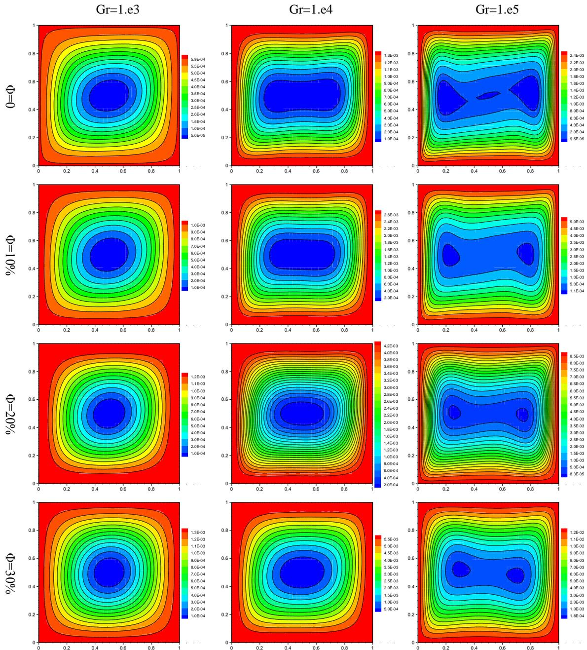
Figure (5)- Streamlines contours for Cu-water nanofluids at various Grashof numbers and volume fraction
