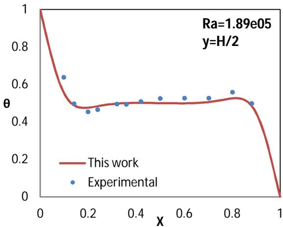
Figure (3)- Comparison of the temperature profiles between the present results and the experimental results by Krane and Jessee ( $Ra=1.890 \times 10^5$ ,  $Pr=0.71$ )
