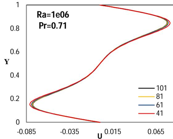
Figure (2)- Horizontal velocity profiles at mid-sections of the cavity for various mesh sizes
