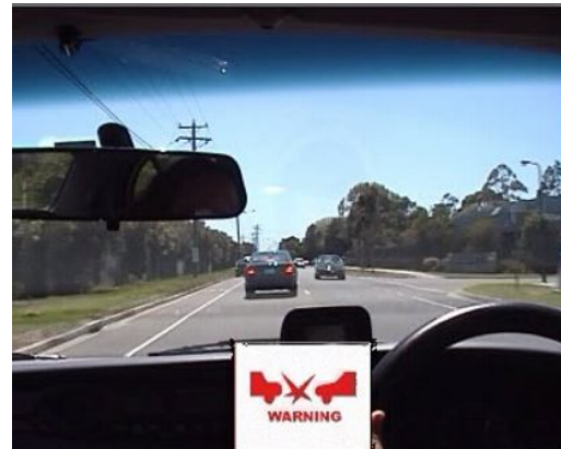
Figure.2. Forward Collision Warning
