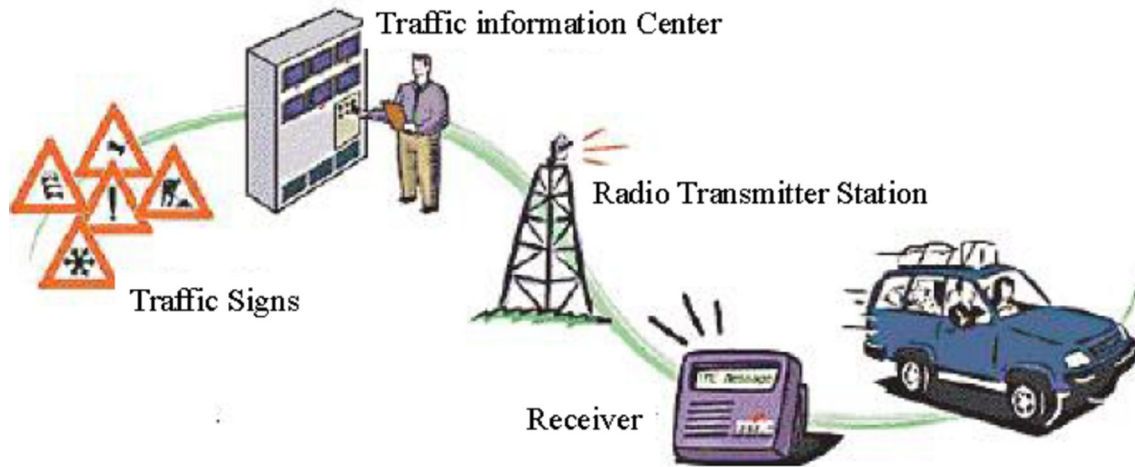
Figure1. Components of a road information system
