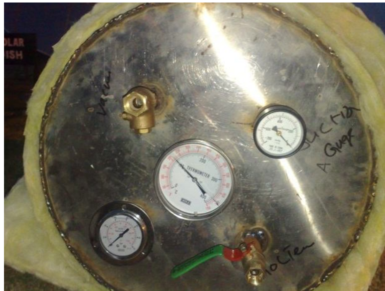
Fig. 5. Battery with Insulation and Guages
