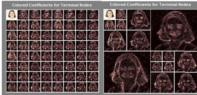
Figure 4. (a) Complete wavelet packets tree. (b) Corresponding best nodes on the base of entropy. These best nodes are used for signatures generation
