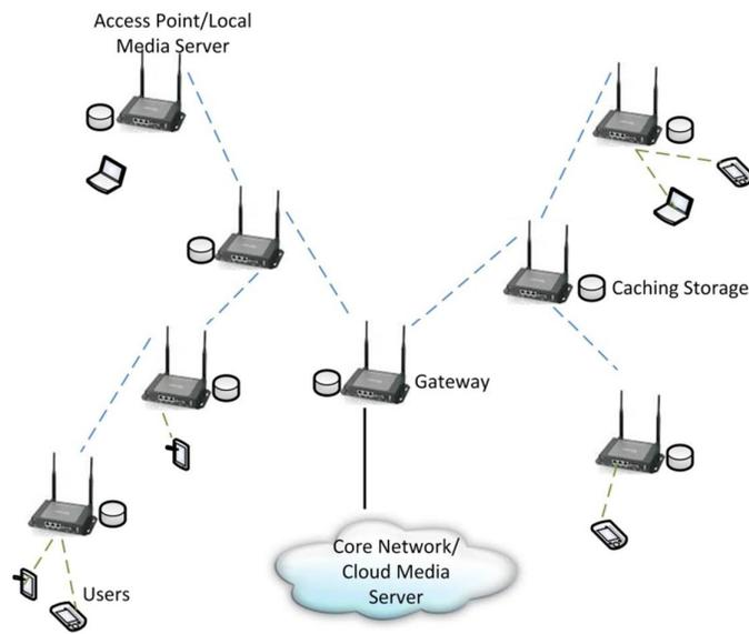
Figure 2. Wireless CDN based on mesh Wi-Fi [20]
