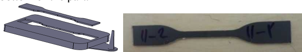
Figure. 4. a schematic test specimen that was cut from the bottom of the part.
