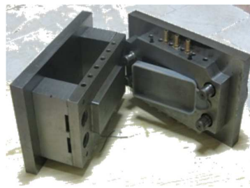
Figure.2. The manufactured mold and injection part.
