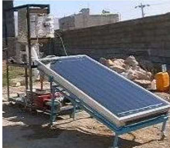
Fig 3. Usage of TCAC in a packed bed dryer
