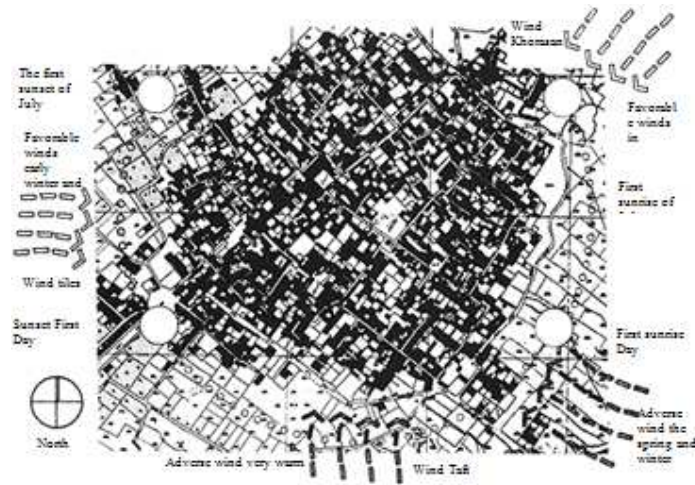
Map1. The arrangement texture map of the path of the sun in winter and summer and favorable and unfavorable wind conditions in different seasons Source: GHOBADIAN 1384
