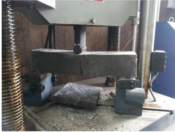
Fig. 4. Flexural specimen failure under the three-point test
