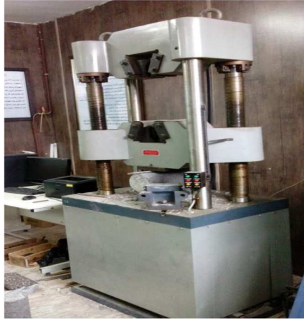
Fig. 3. Apparatus for determining the tensile strength and the specimen below its jack
