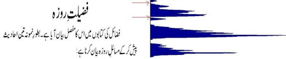
Figure 2: Multiple peaks and valleys in same line of text due to dots and diacritics
