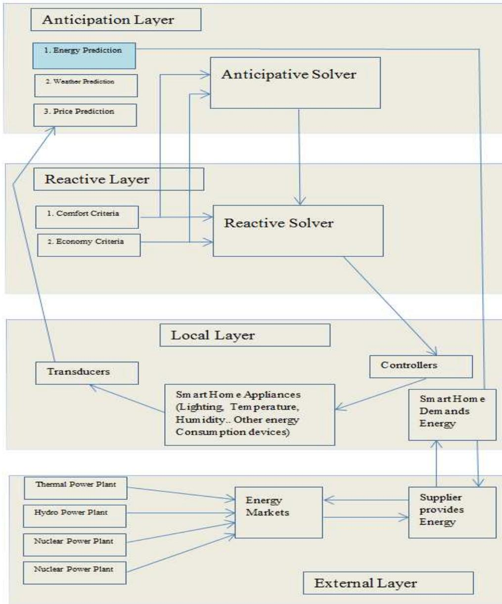
**Figure 2:** Interaction among different components in energy management system
